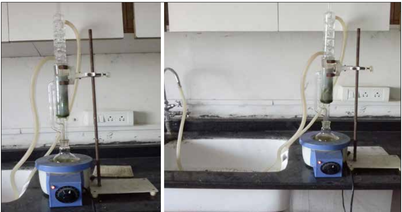
fig. 25a-b Soxhlate apparatus (left); and process of making extract from leaves of Karanj tree (right)
